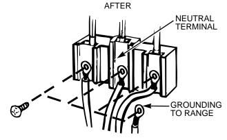
WARNING: THE NEUTRAL WIRE OF SUPPLY CIRCUIT IS CONNECTED TO THE NEUTRAL TERMINAL LOCATED IN THE CENTER OF THE CONNECTOR BLOCK. THE POWER LEADS MUST BE CONNECTED TO THE OUTSIDE (BRASS COLORED) TERMINALS. THE 4TH GROUNDING LEAD MUST BE CONNECTED TO THE FRAME OF THE RANGE WITH THE GROUNDING SCREW.
